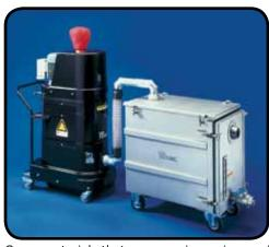
Ruwac's portable immersion separation systems are designed to safely collect explosive or glowing media by capturing the hazardous material and completely submerging it in liquid. The chance of an outside ignition source entering the vacuum, is safely ruled out.
